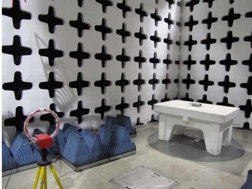
Photo 1. Radiated emissions test setup with Loop antenna.
