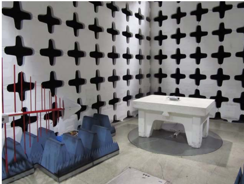
Photo 2. Radiated emissions test setup with Biconilog antenna.
