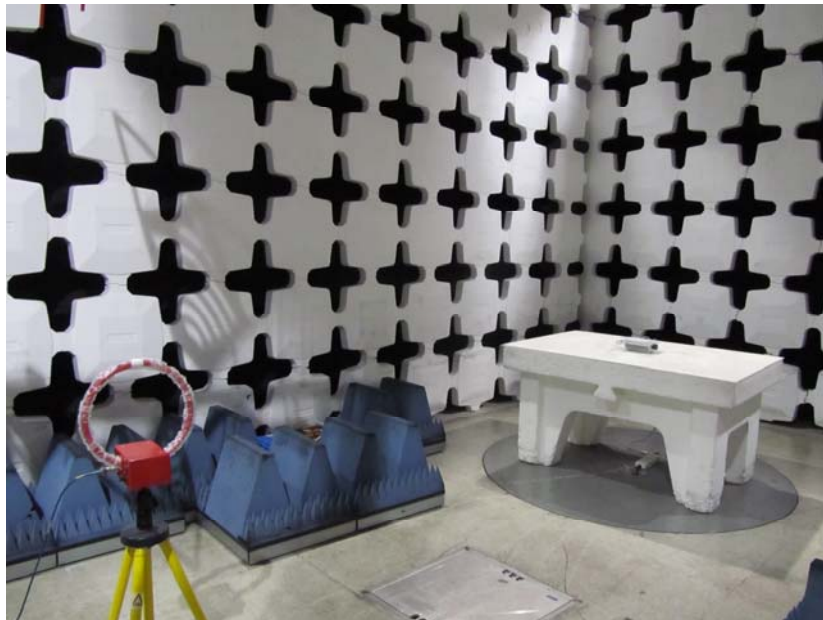
Photo 1. Radiated emissions test setup with Loop antenna.
