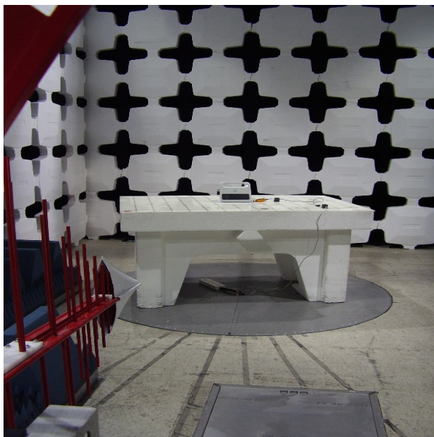
Photo 2. Radiated emissions test setup with Biconilog antenna.
