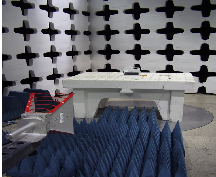
Photo 3. Radiated emissions test setup with Horn antenna.
