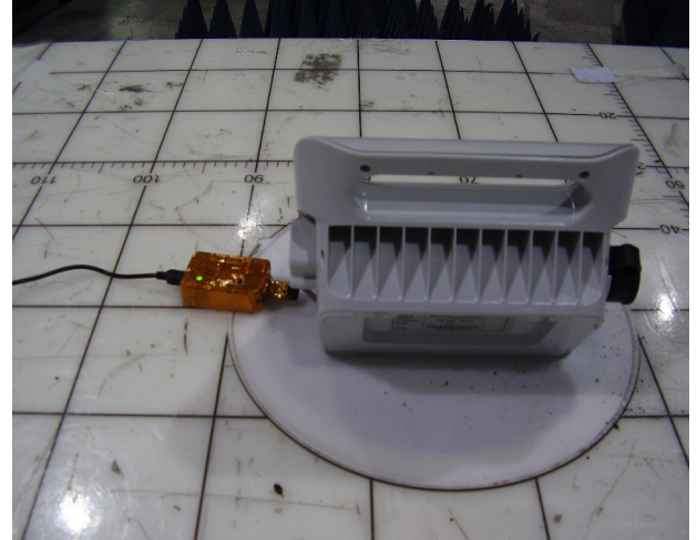
Photo 6. Radiated emissions test setup rear view.
