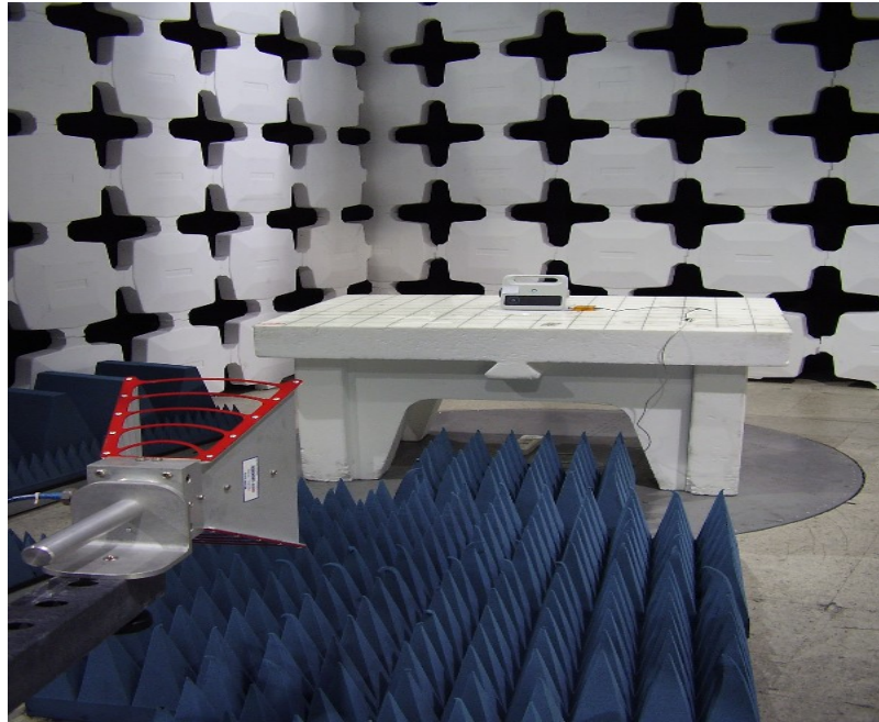
Photo 3. Radiated emissions test setup with Horn antenna.
