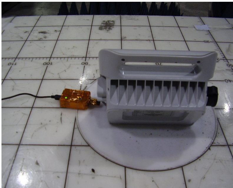
Photo 6. Radiated emissions test setup rear view.
