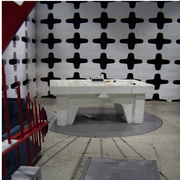
Photo 2. Radiated emissions test setup with Biconilog antenna.
