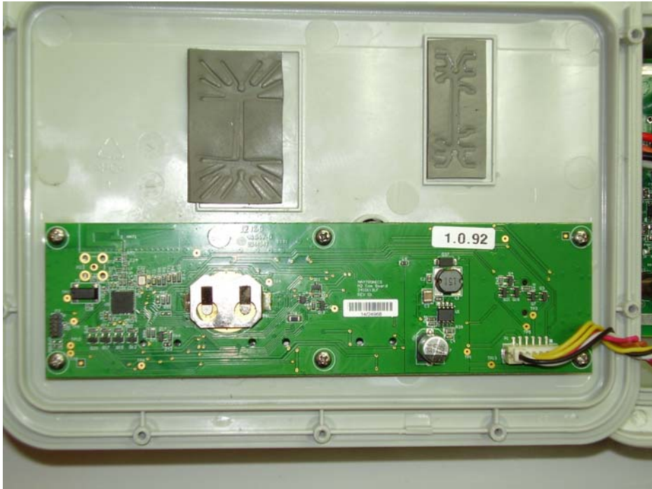
The Transceiver Module position into the auxiliary equipment. RF board only
