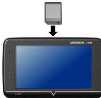
To remove a card, gently push the top edge of the card inwards to release it, and pull it out of the slot.
