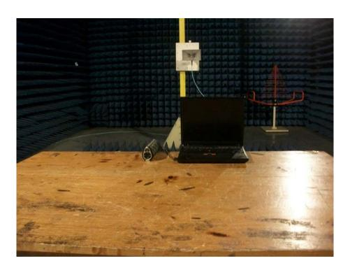
SPURIOUS EMISSION TEST SETUP
