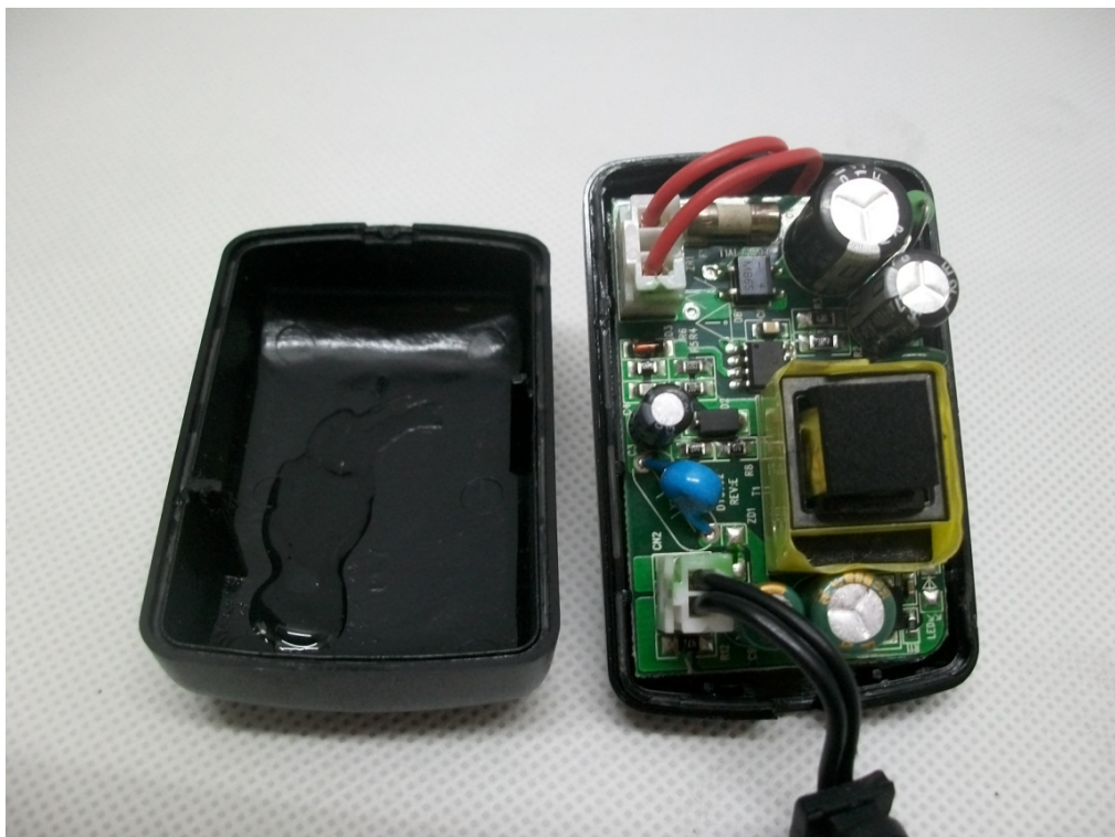
INTERNAL PHOTO OF POWER SUPPLY1 - 1
