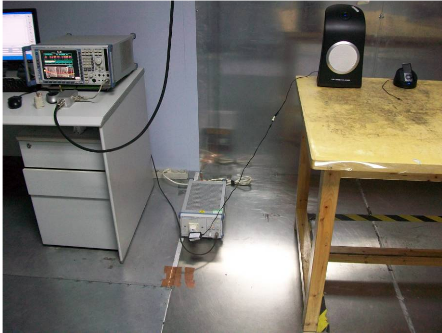
Photograph- Test Setup for Conducted Emission
