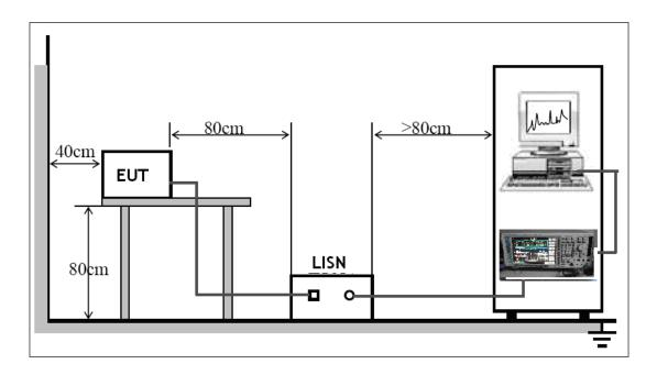
The EUT was placed on the test table in shielding room
