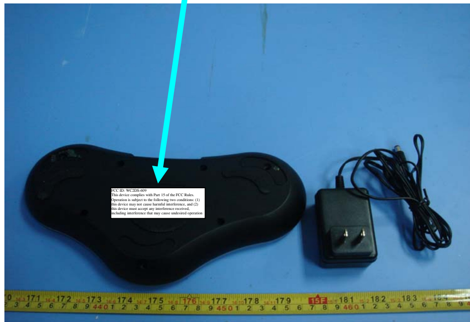
Proposed Label Location on EUT EUT Bottom View/proposed FCC Mark Location
