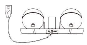
2. Plug the AC adaptor into the DC in port at the rear of the base station, then into a power supply.(100-240V/50Hz AC electrical outlet)
