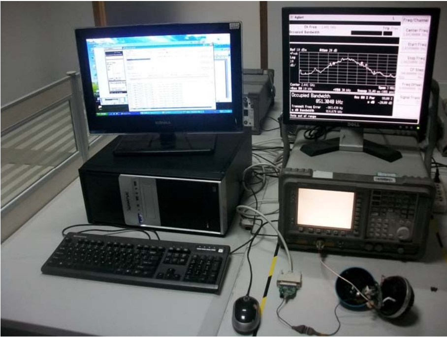
SPURIOUS EMISSION TEST SETUP
