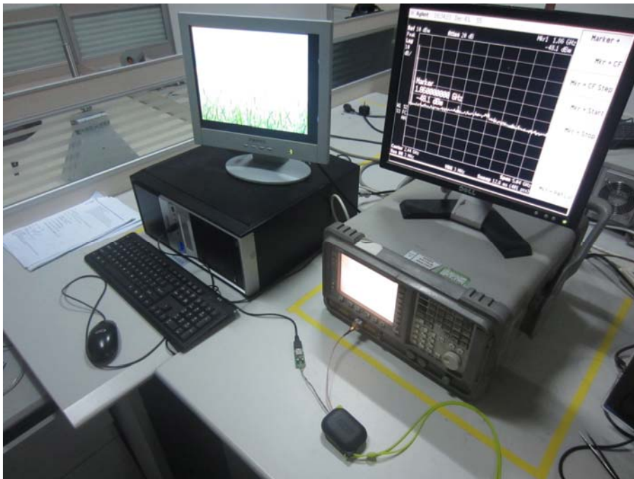
SPURIOUS EMISSION TEST SETUP
