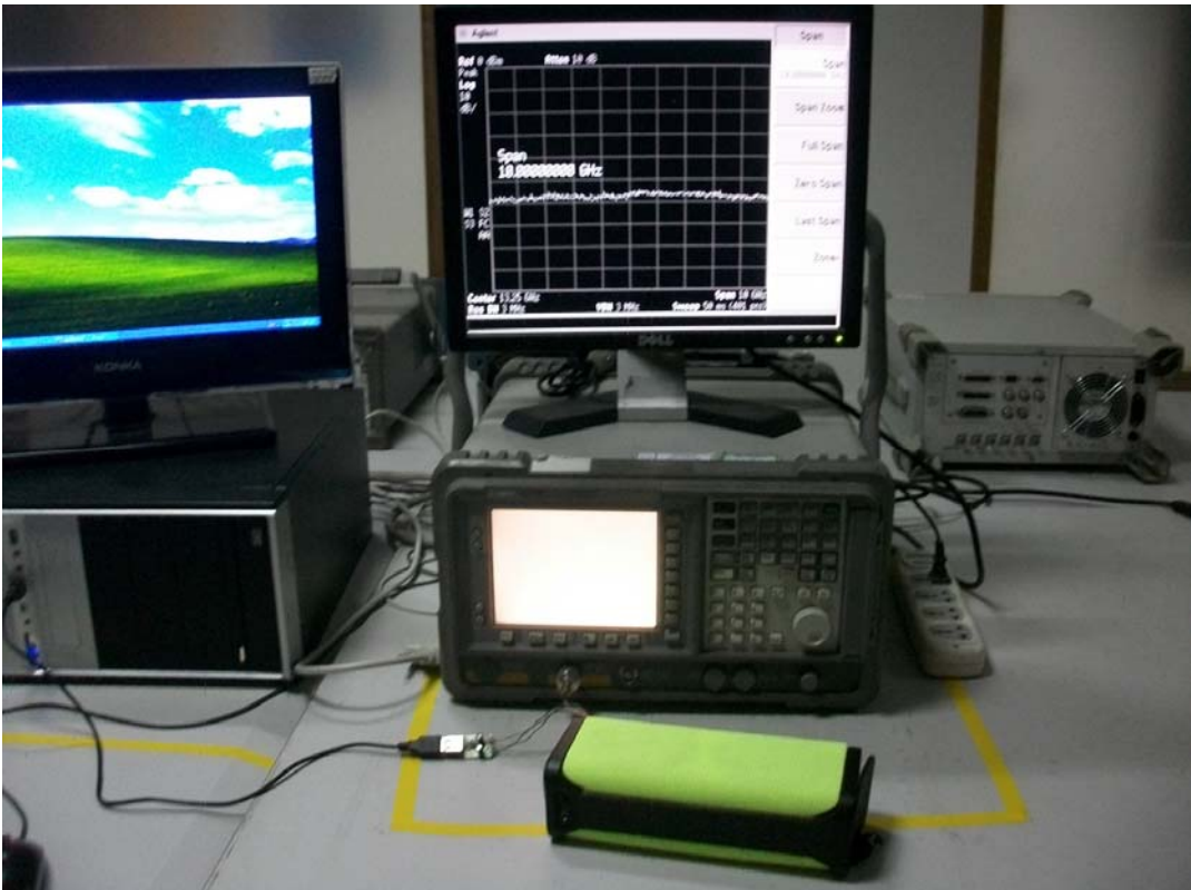
SPURIOUS EMISSION TEST SETUP
