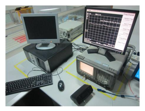
CONDUCTED EMISSION TEST SETUP
