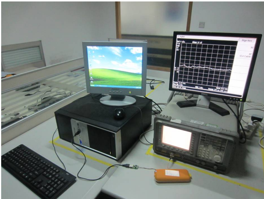
SPURIOUS EMISSION TEST SETUP
