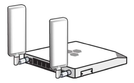
Aerohive BR200-LTE-VZ routers allow enterprises to provision branch office networks and teleworkers quickly and easily. The BR200-LTE-VZ router provides LAN and WLAN connectivity and PoE (power over Ethernet) support.
