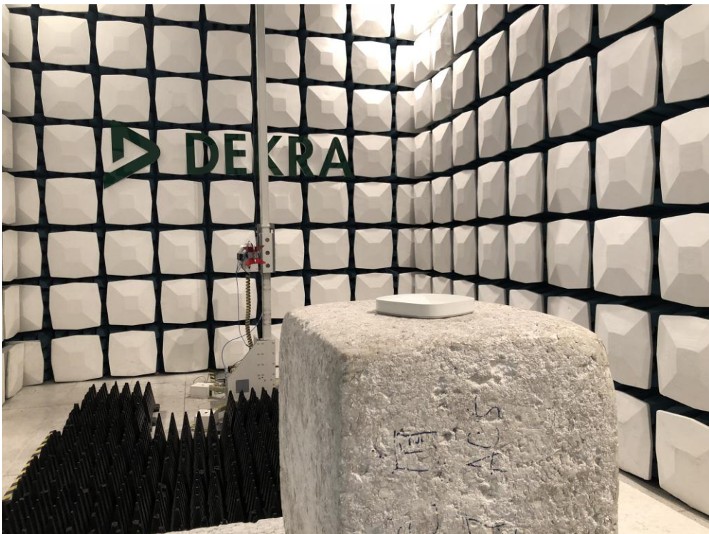
Description: Radiated Emission Test Setup for 1~18GHz
