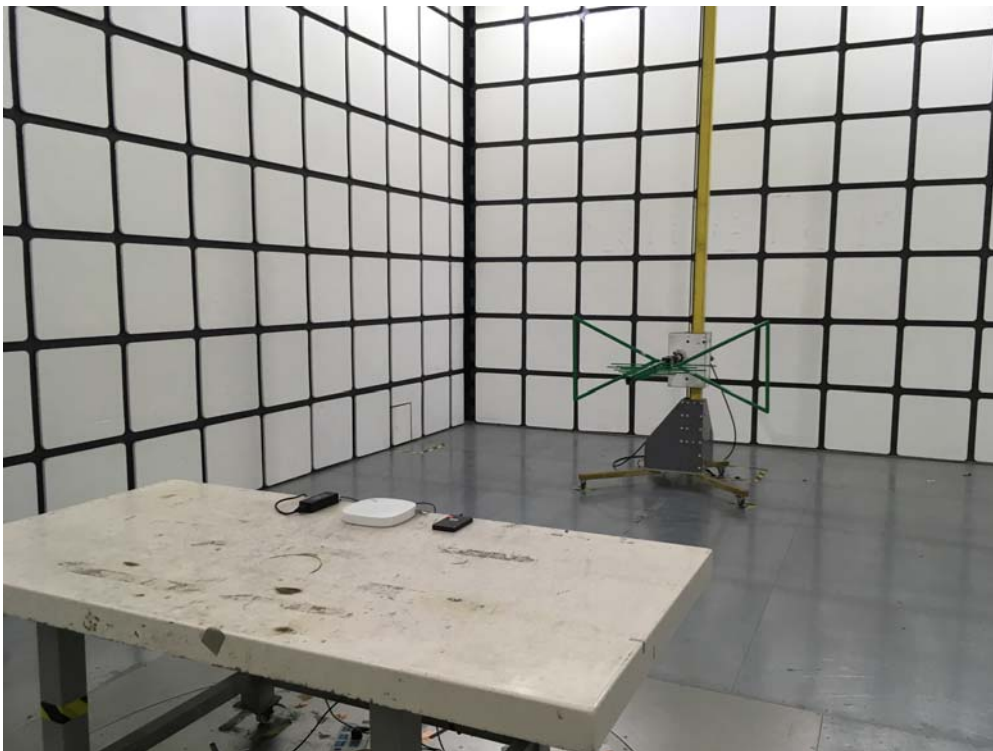
Description: Radiated Emission Test Setup for 1~18GHz
