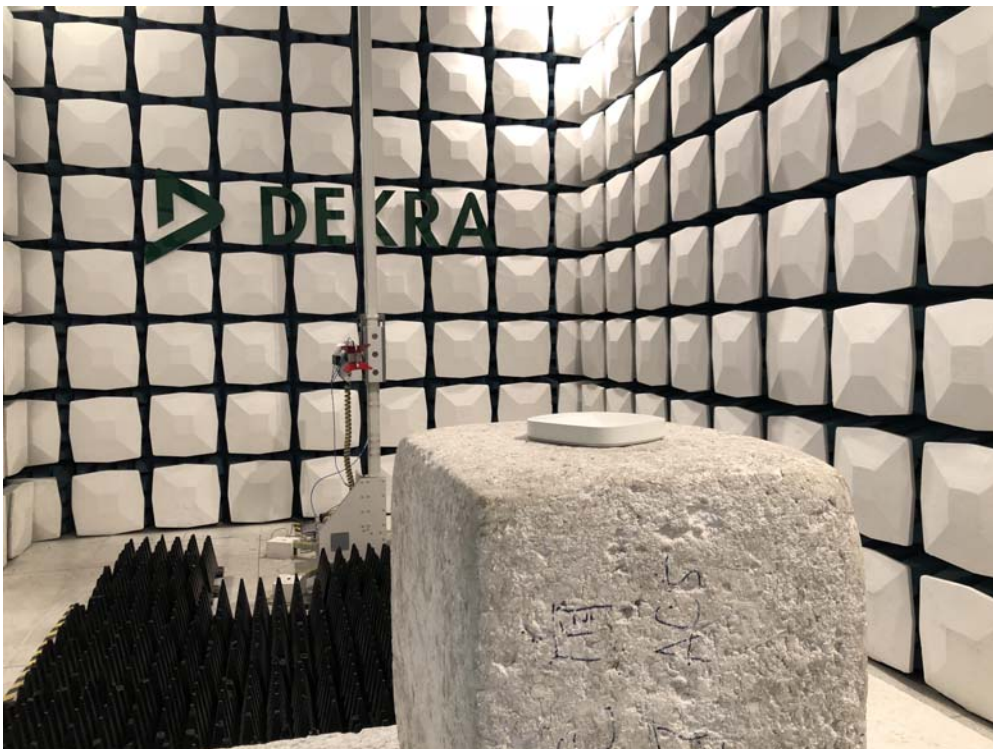
Description: Radiated Emission Test Setup for 1~18GHz
