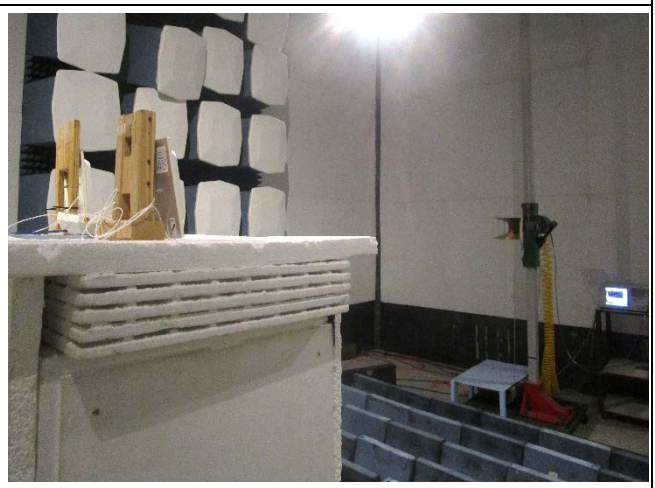
Radiated Emissions (>1GHz) – Rear View
