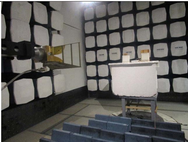
Radiated Emissions (>1GHz) – Front View
