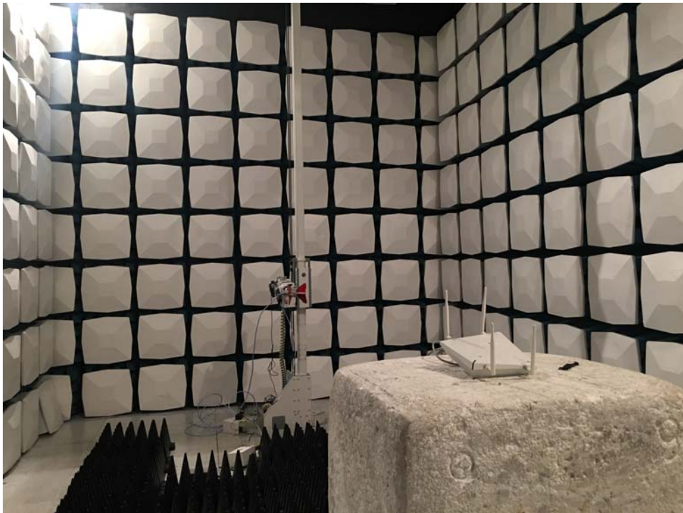
Description: Radiated Emission Test Setup for 1~18GHz
