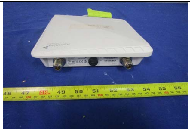
Access Point - Rear View
