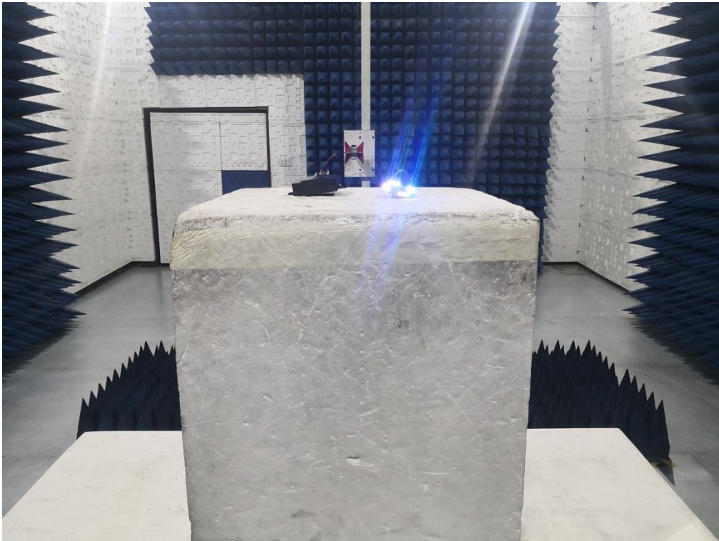
RADIATED EMISSION TEST SETUP ABOVE 1GHZ
