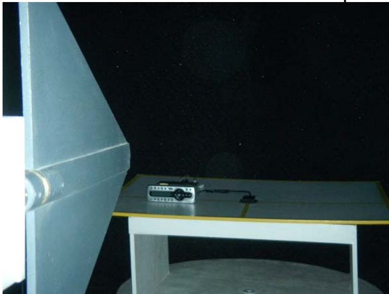
Measurement of Radiated Emission Test Set up
