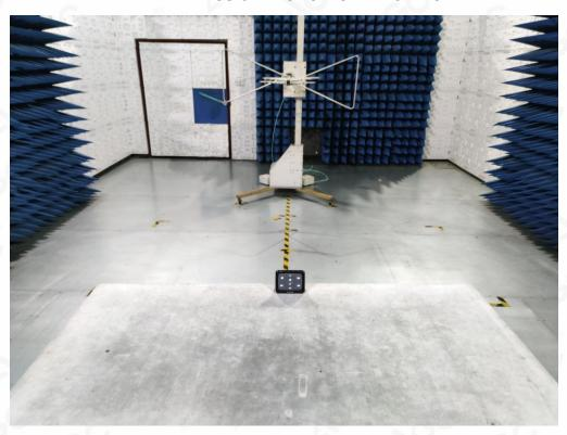
RADIATED EMISSION TEST SETUP ABOVE 1GHz
