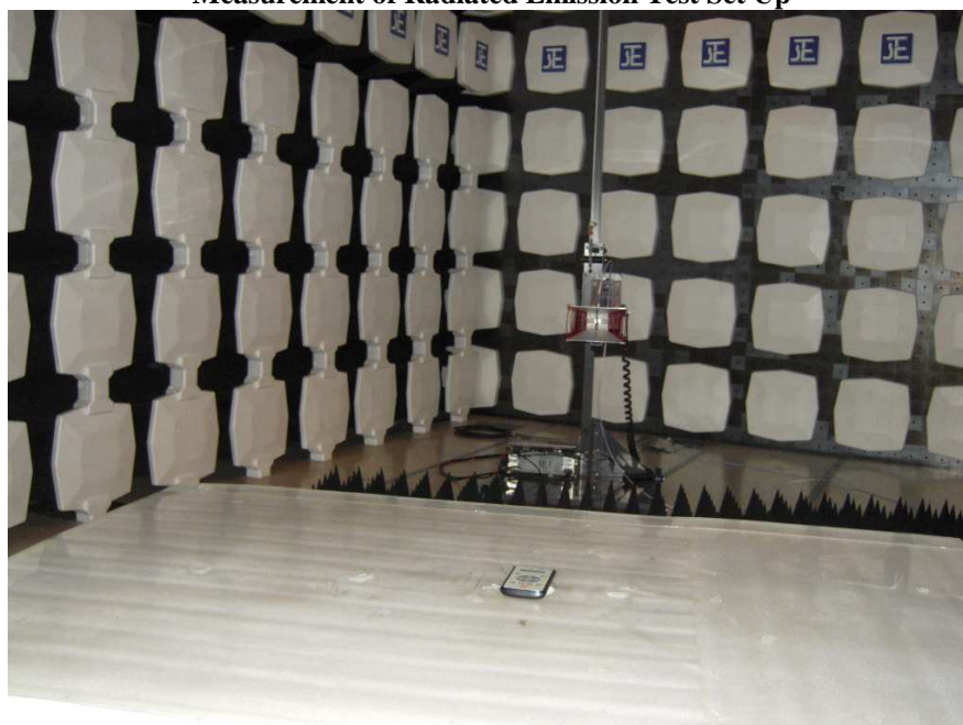
Measurement of Radiated Emission Test Set Up
