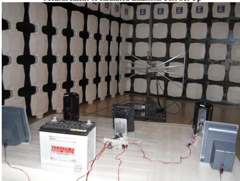
Measurement of Radiated Emission Test Set Up
