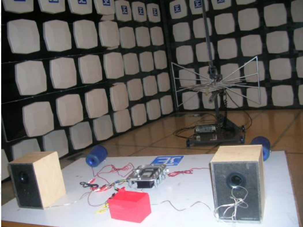
Measurement of Radiated Emission Test Set Up
