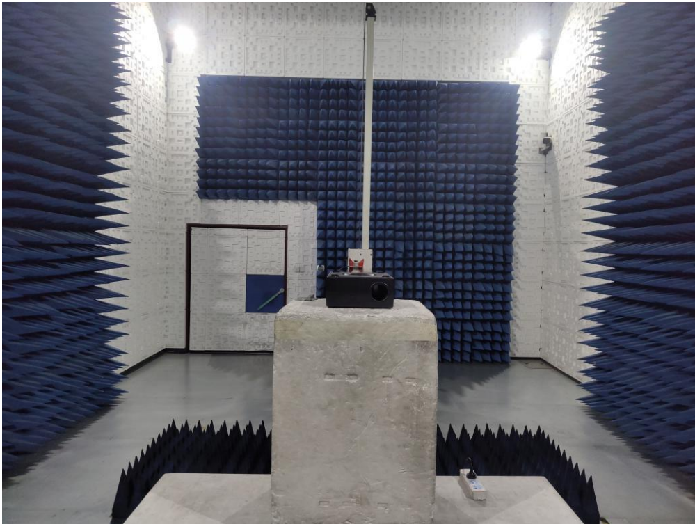
RADIATED EMISSION TEST SETUP ABOVE 1GHz
