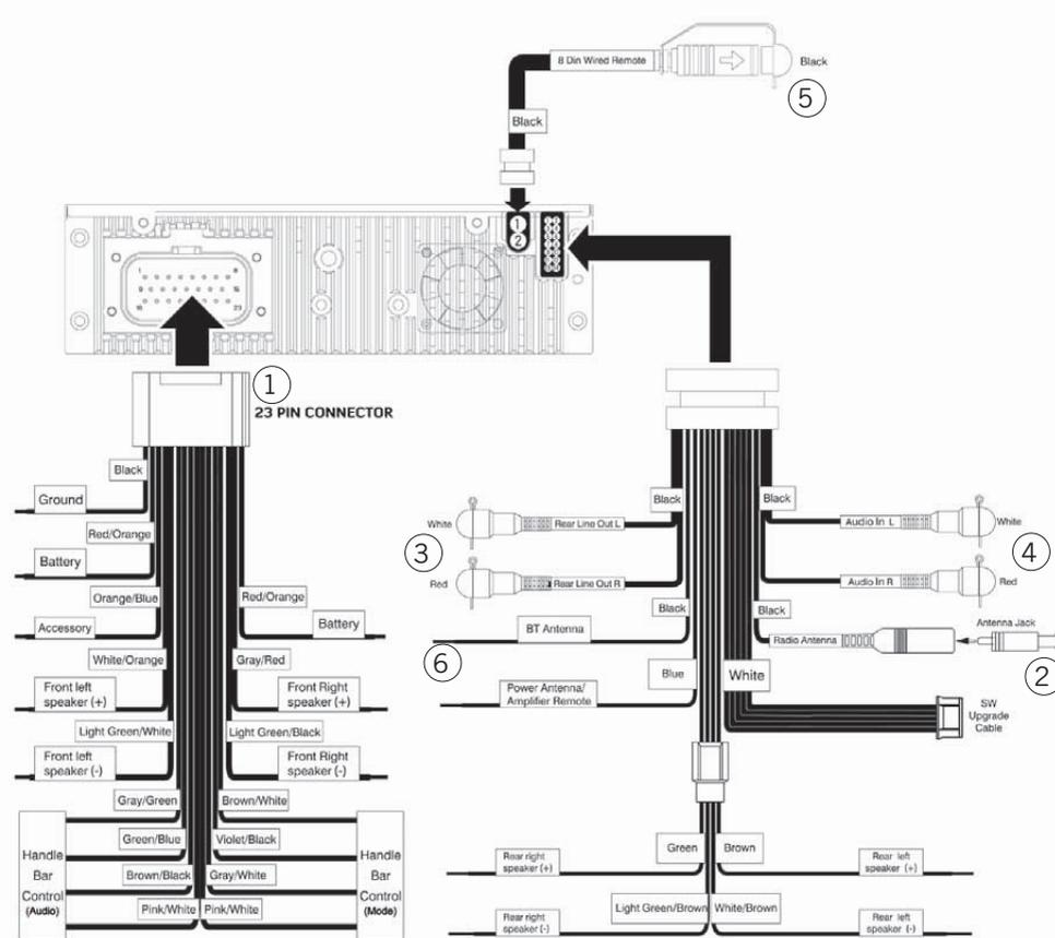
**⚠** No lower than a 2 Ohm load should be used or damage may occur to the Media Player. Make sure the polarity of speakers are connected correctly.
