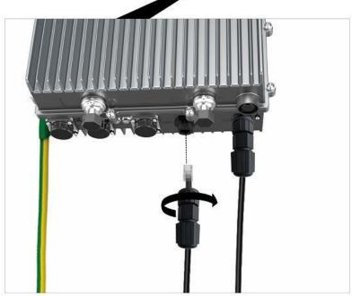
Connect and tighten the waterproof cable (\*\sum waterproof sleeve to be purchased separately) to MP-PS.
