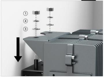
Hang the MP-PS on the mounting bracket  $\,\mathrm{I}$  and fasten with  $\,2{\times}M10$  nuts.
