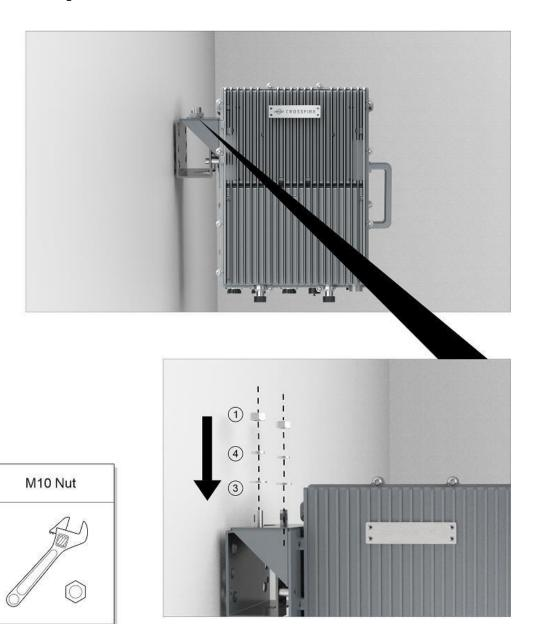
Hang the MP-PS on the mounting bracket  $\,I$  and fasten with  $\,2{\times}M10$  nuts.
