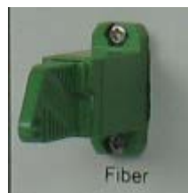
Figure 23 E2000 Fiber Optic Port on Host Unit FIU
