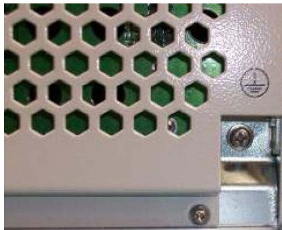
Figure 19 Host Unit Grounding Stud
