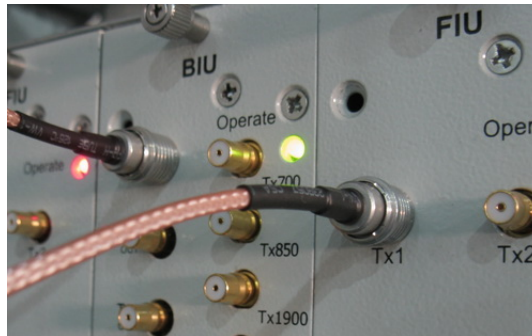
Figure 21 BTS QMA Coaxial Cable Connection
