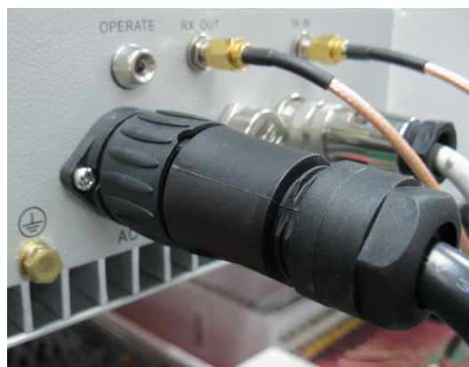
Figure 364-Pin AC Power Connector
