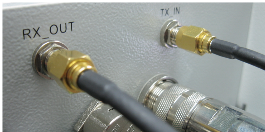
SMA Coaxial Cable Inter-connection on Single-band Enclosure
