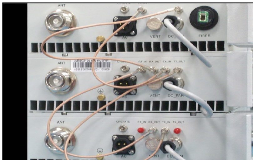
Figure 4-13. RF cable connection between Slave to Slave Remote Units
