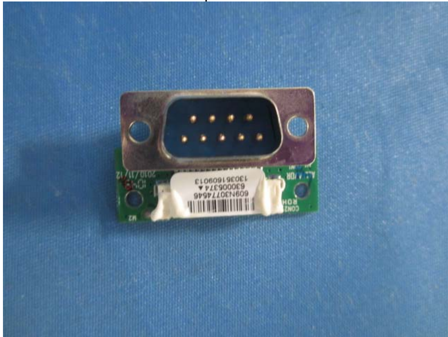
Control port front view
