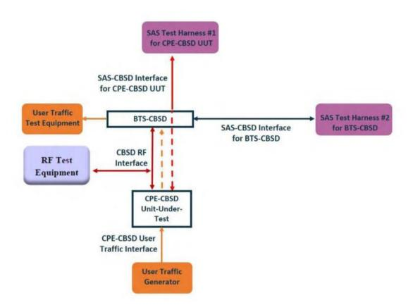
Test setup diagram for WINNF.PT.C.HBT Test case
