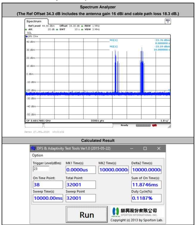
The sum of On Time (aggregated time from marker 1 to 2): 11.87ms < 1s, Pass.
