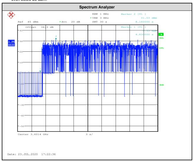
Note: The Ref Offset 34.3 dB includes the antenna gain 16 dBi and cable path loss 18.3 dB.
