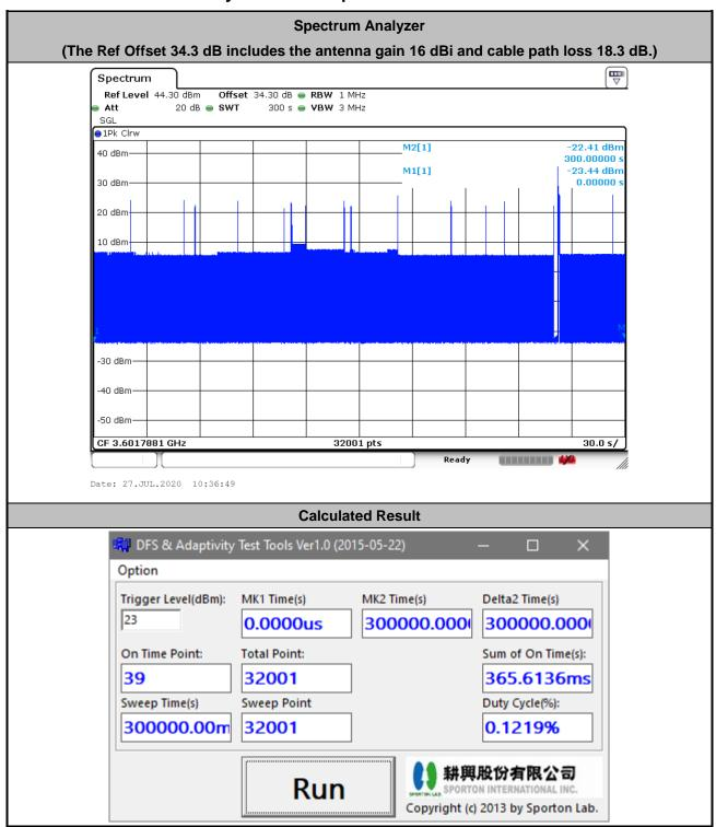
The sum of On Time (aggregated time from marker 1 to 2): 365.61ms < 10s, Pass.
