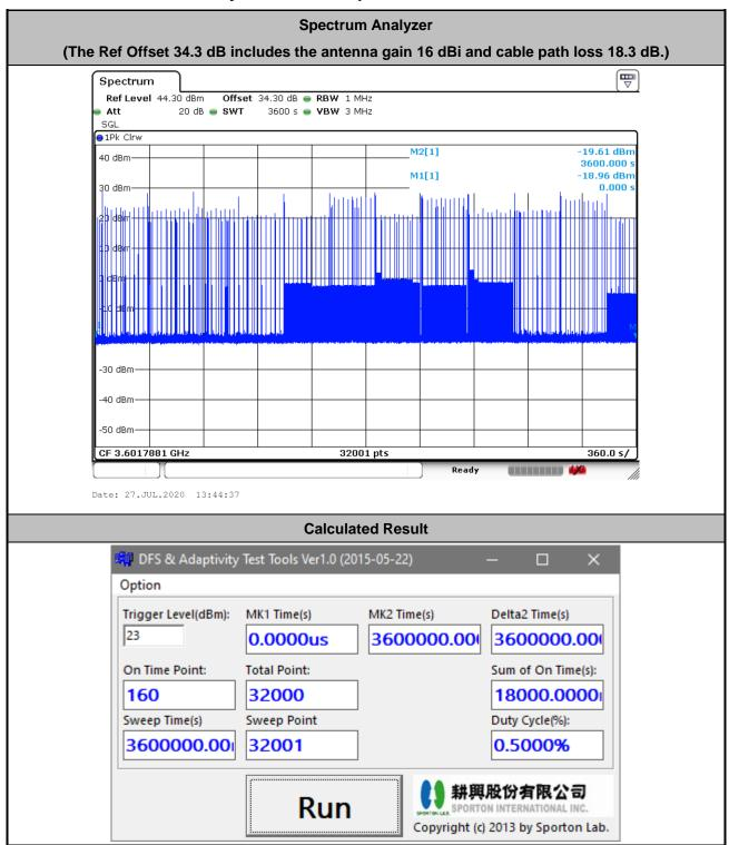
The sum of On Time (aggregated time from marker 1 to 2): 18s < 20s, Pass.
