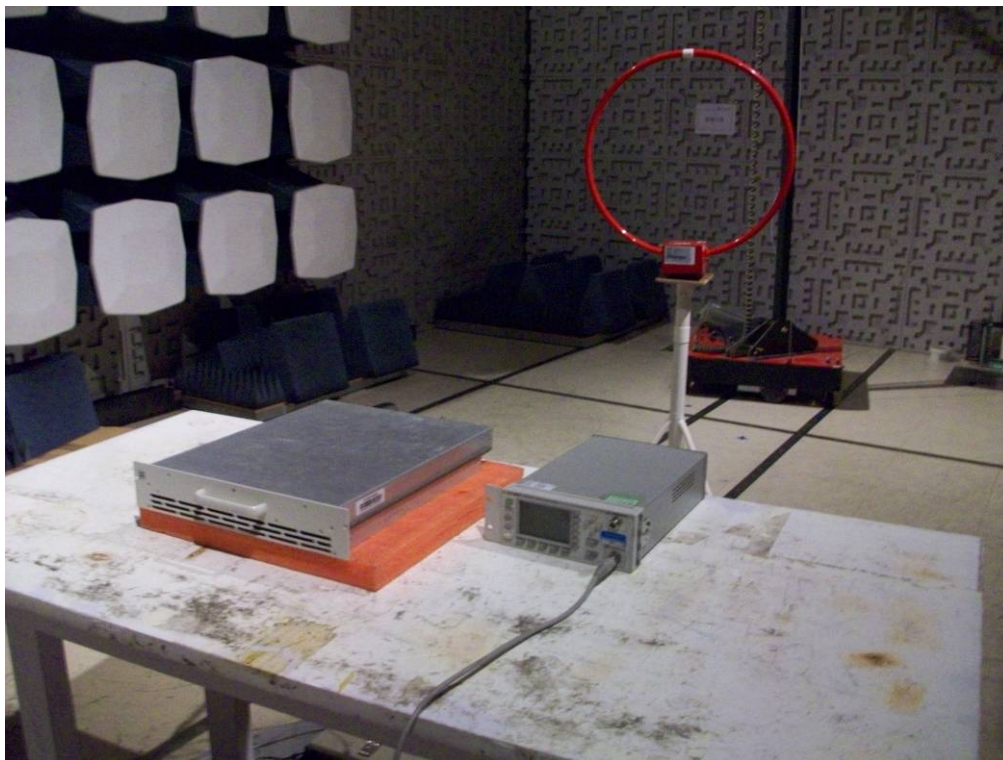
TEST SETUP OF RADIATED EMISSION (9kHz-30MHz)
