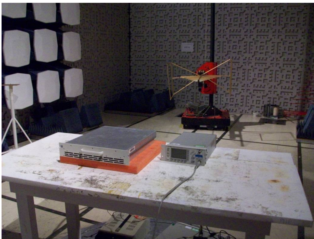
TEST SETUP OF RADIATED EMISSION (30MHz-1GHz)
