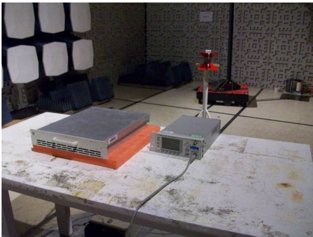
TEST SETUP OF RADIATED EMISSION (above 1GHz)
