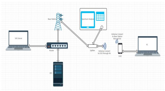
Test setup diagram for WINNF.PT.C.HBT Test case
