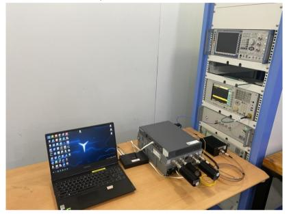
Radiated Spurious Emissions (30MHz-1GHz)
