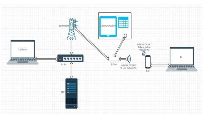
Test setup diagram for WINNF.PT.C.HBT Test case
