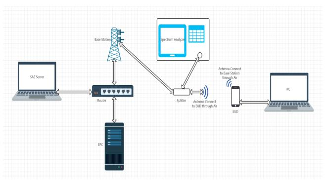
Test setup diagram for WINNF.PT.C.HBT Test case
