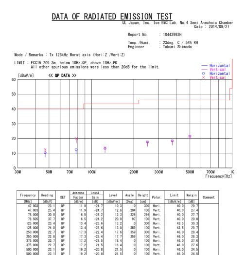
CHART:WITH FACTOR ANT TYPE: -30MHz:LOOP, 30-300MHz:BICONICAL, 300MHz-1000MHz:LOGPERIODIC, 1000MHz-:HORN CALCULATION:RESULT = READING + ANT FACTOR + LOSS(CABLE + ATTEN. - GAIN(AMP))
