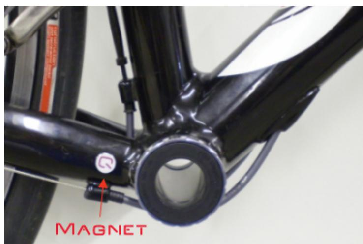
The CinQo's cadence sensors are located on the back of the CinQo under the five bumps. The CinQo is supplied with a neodymium magnet and 3M dual sided adhesive. The magnet should be in line with the cadence sensors and within  $\frac{1}{2}$  inch (12 mm) from the sensors. Do not allow the magnet to physically touch the sensors.
