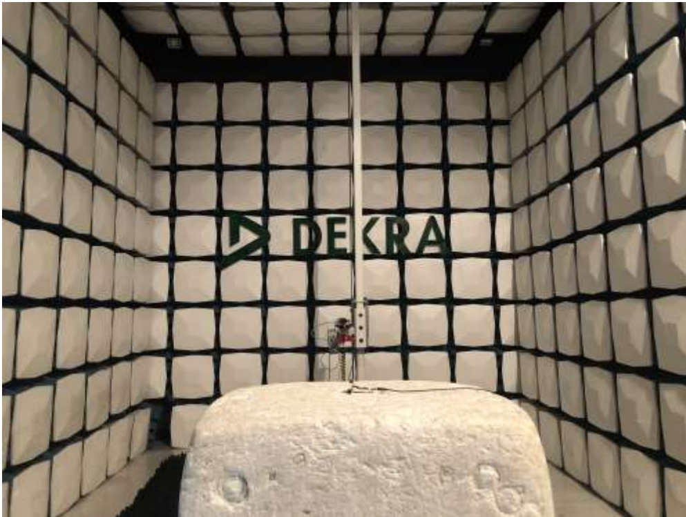
Description: Radiated Emission Test Setup for 1~18GHz
