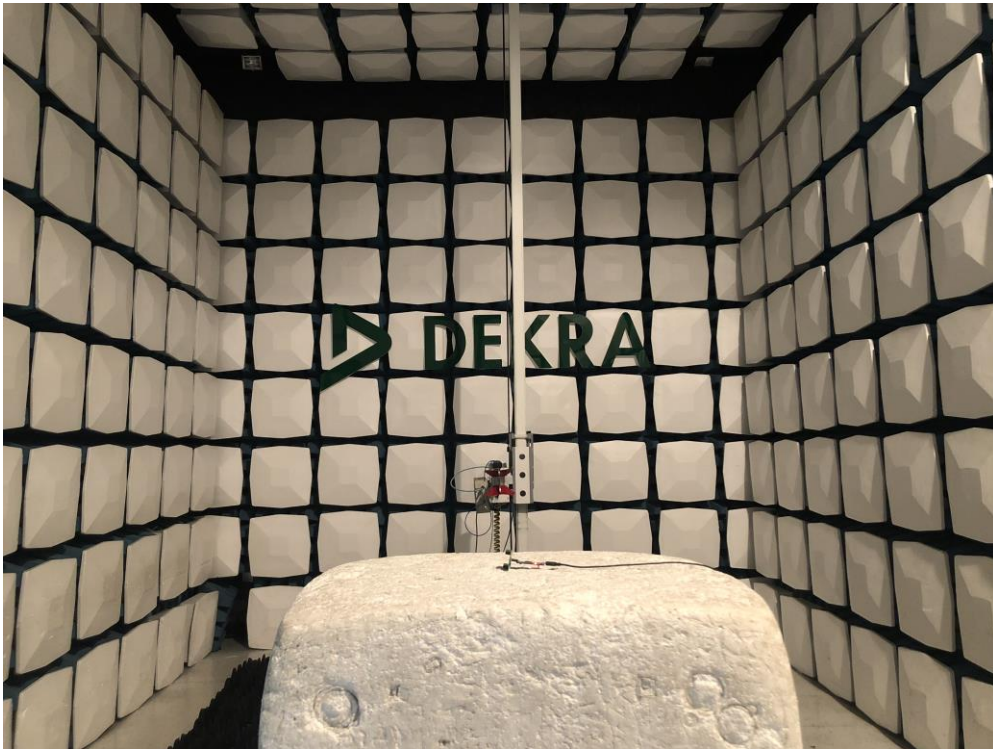
Description: Radiated Emission Test Setup for 1~18GHz
