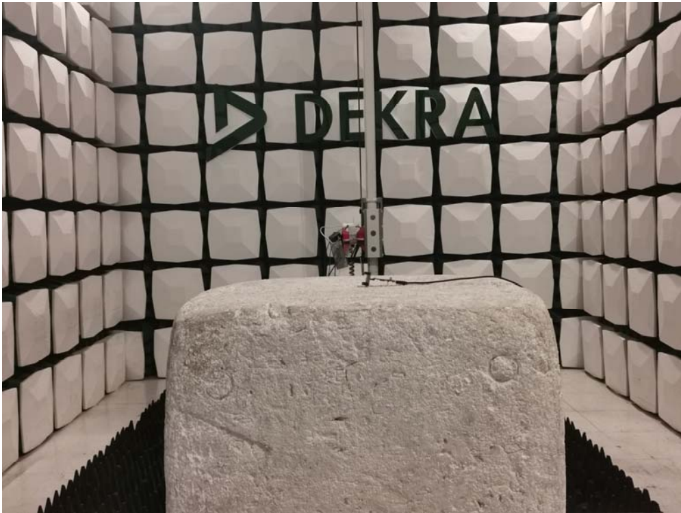
Description: Radiated Emission Test Setup for 1~18GHz
