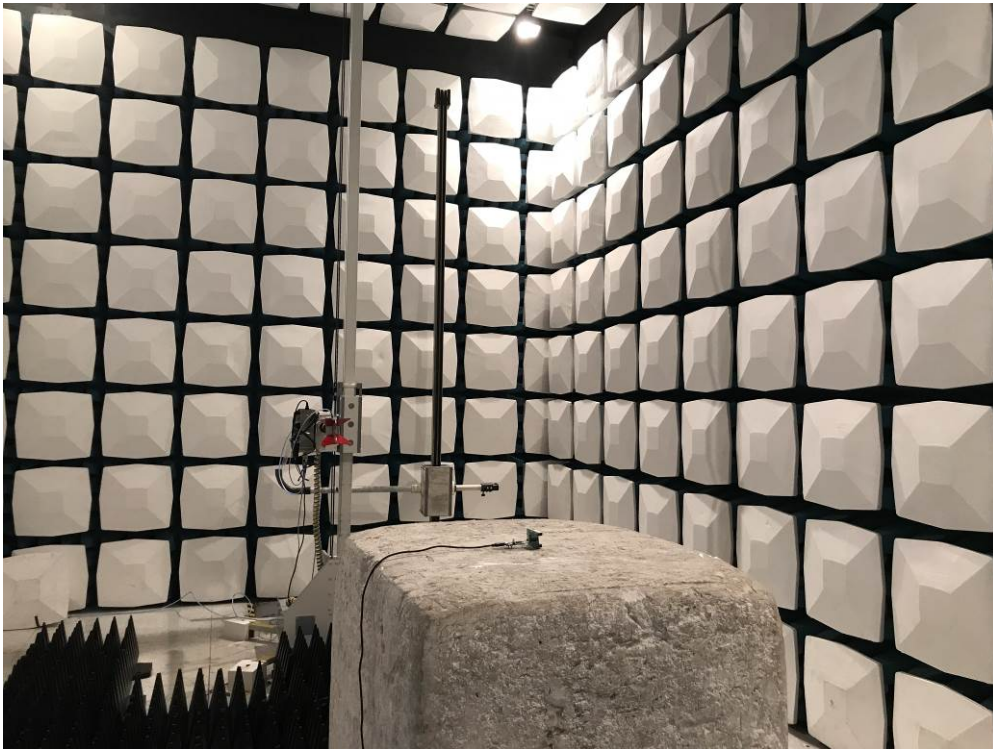
Description: Radiated Emission Test Setup for 1~18GHz
