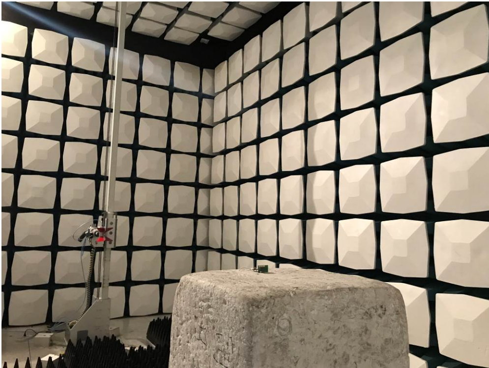
Description: Radiated Emission Test Setup for 1~18GHz
